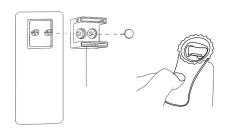
Insert back of wall bracket into place (Top of wall bracket has key holes)
